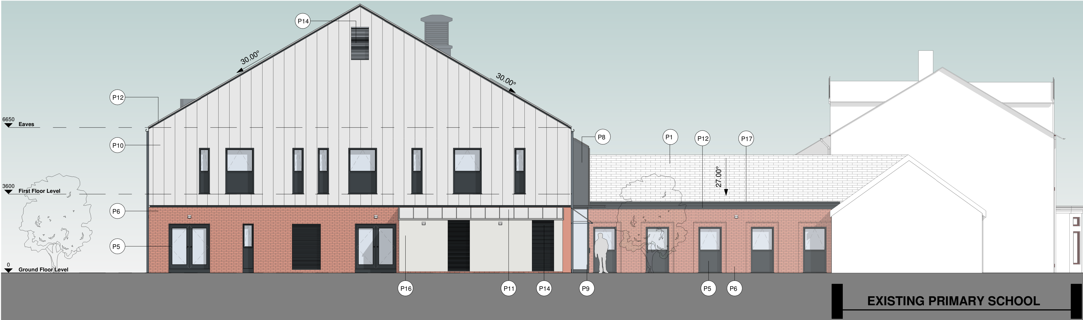
3 21ZZ_North - West Elevation as Proposed 1 : 100
