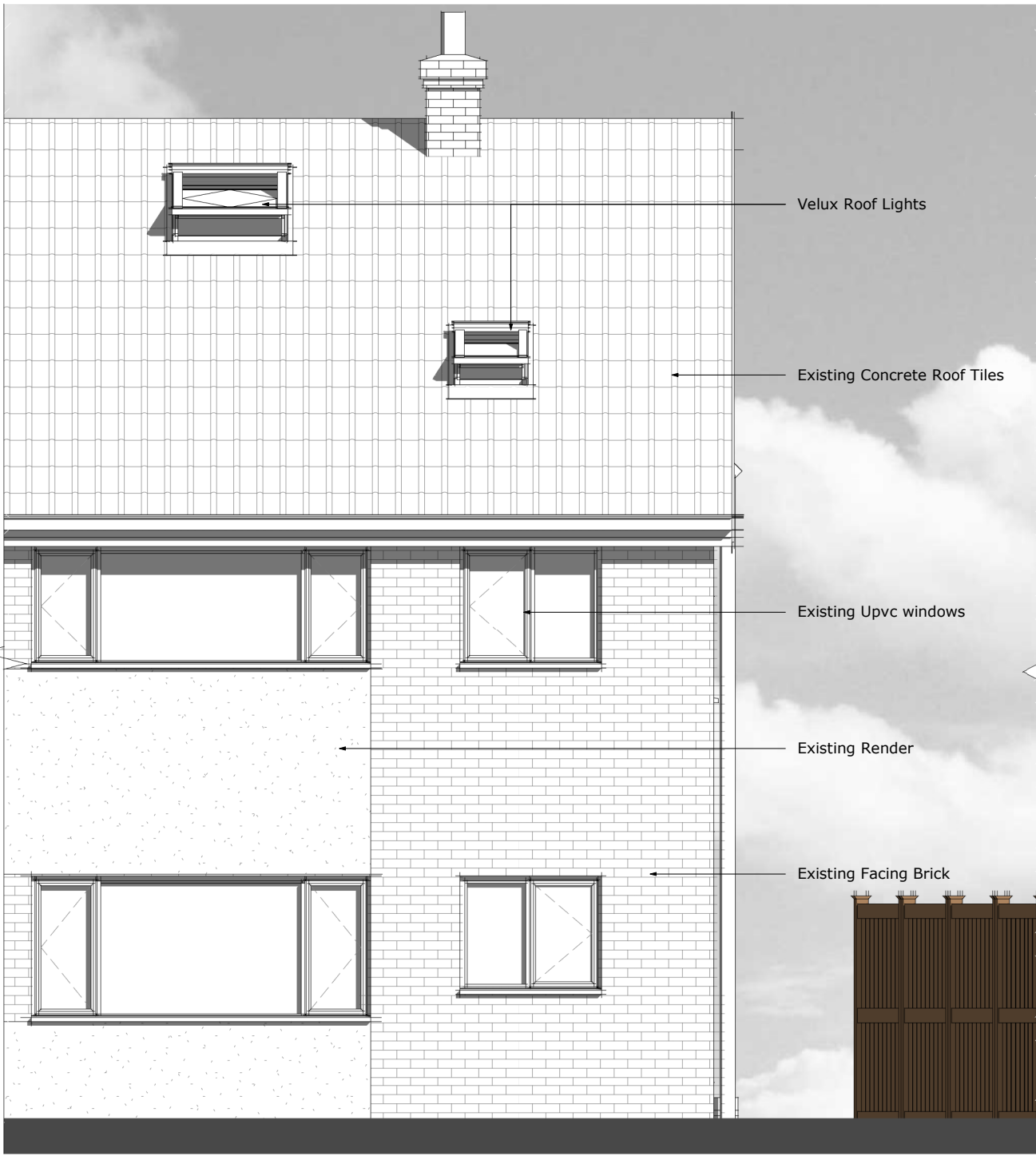
4 Existing Rear Elevation - North
