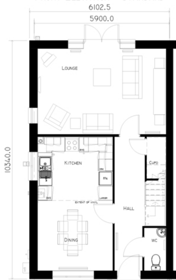
GROUND FLOOR PLAN GFA 53.96M 2 (53.05M 2 )
