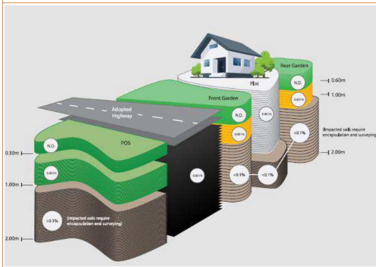
FIGURE 4.1 ASBESTOS RISK MITIGATION CONCEPTUAL SITE MODEL
