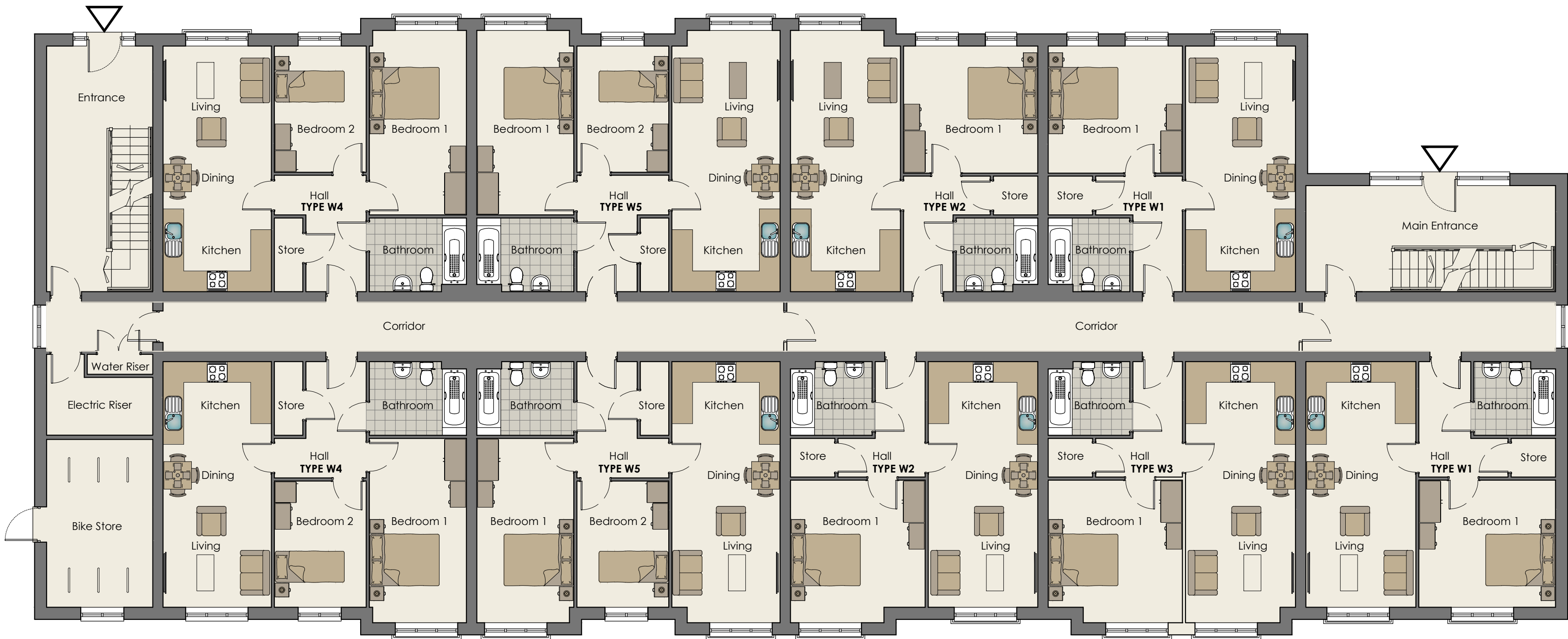
TYPE W - APARTMENTS GROUND FLOOR PLAN
