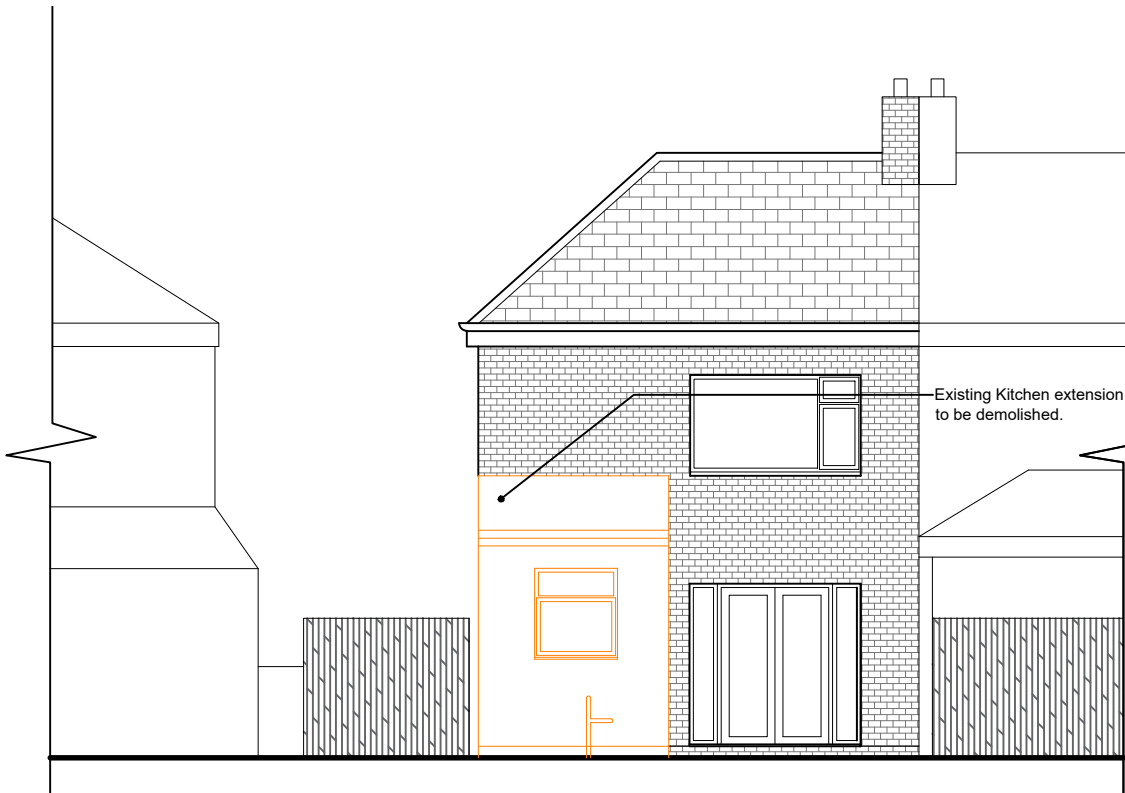
DEMOLITION ELEVATION C-C SCALE 1:100
