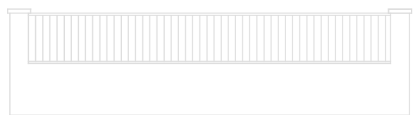
B - B - Denotes 2m high brick and wooden panel wall
