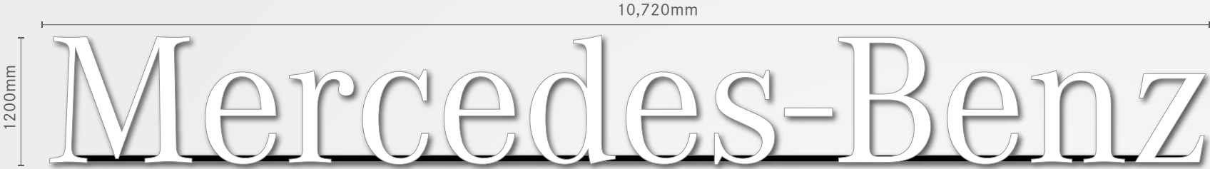
Item A - 380 1no. Sets individual white internally illuminated letters with black runner bars. Scale 1:50
