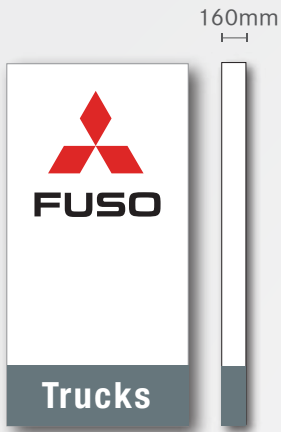
Item H 1no. Single sided internally illuminated sign. Size: 1200mm x 2406mm Scale 1:50
