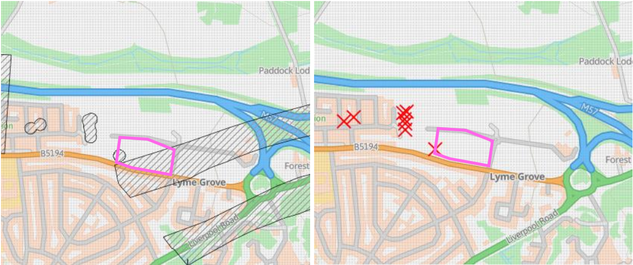
Figure 2 – Mining Remediation Authority Map Extracts Mining Remediation Authority Recorded Development High Risk Area (left) Highlighted in Black Hatching. Mining Remediation Authority Recorded Mine Entries (right) Highlighted by Red X. Approximate Site Boundary in Pink.
