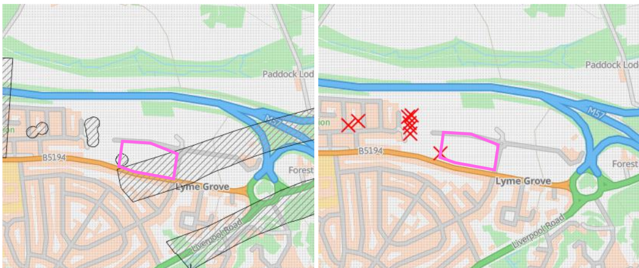
Figure 4 – Mining Remediation Authority Map Extracts Mining Remediation Authority Recorded Development High Risk Area (left) Highlighted in Black Hatching. Mining Remediation Authority Recorded Mine Entries (right) Highlighted by Red X. Approximate Site Boundary in Pink.
