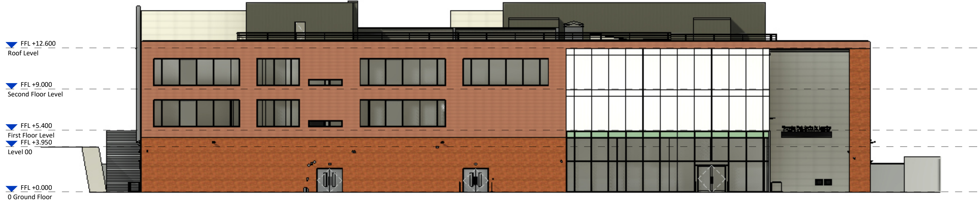
4 Existing West Elevation - Sheet E2002 1 : 200
