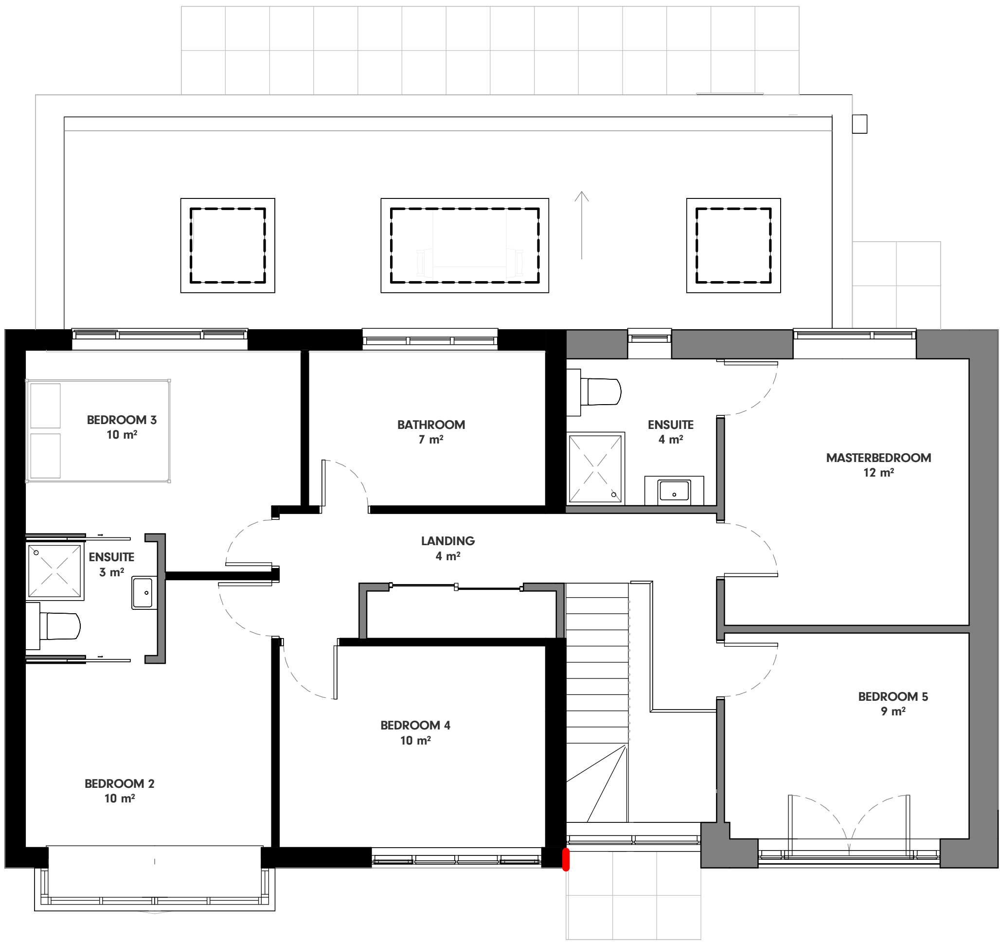
Proposed First Floor Plan 1 : 50
