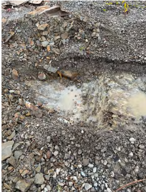
Photo 2: Trial hole showing mudstone at high level. 300 to 400mm below existing surface
