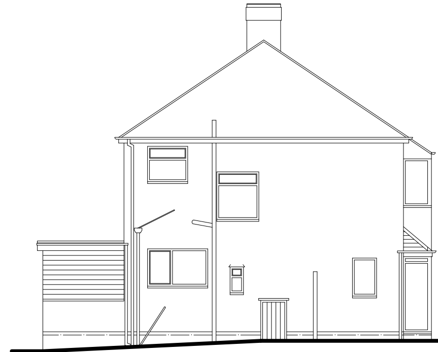
Existing side (north) elevation @ 1:100 scale
