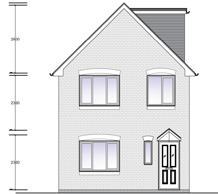
PROPOSED FRONT ELEVATION (Scale 1:100)
