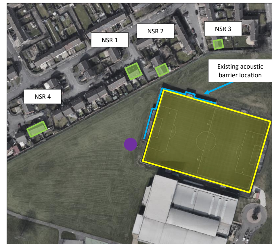
Figure 1: Existing AGP (yellow), with measurement position in purple and existing acoustic barrier
