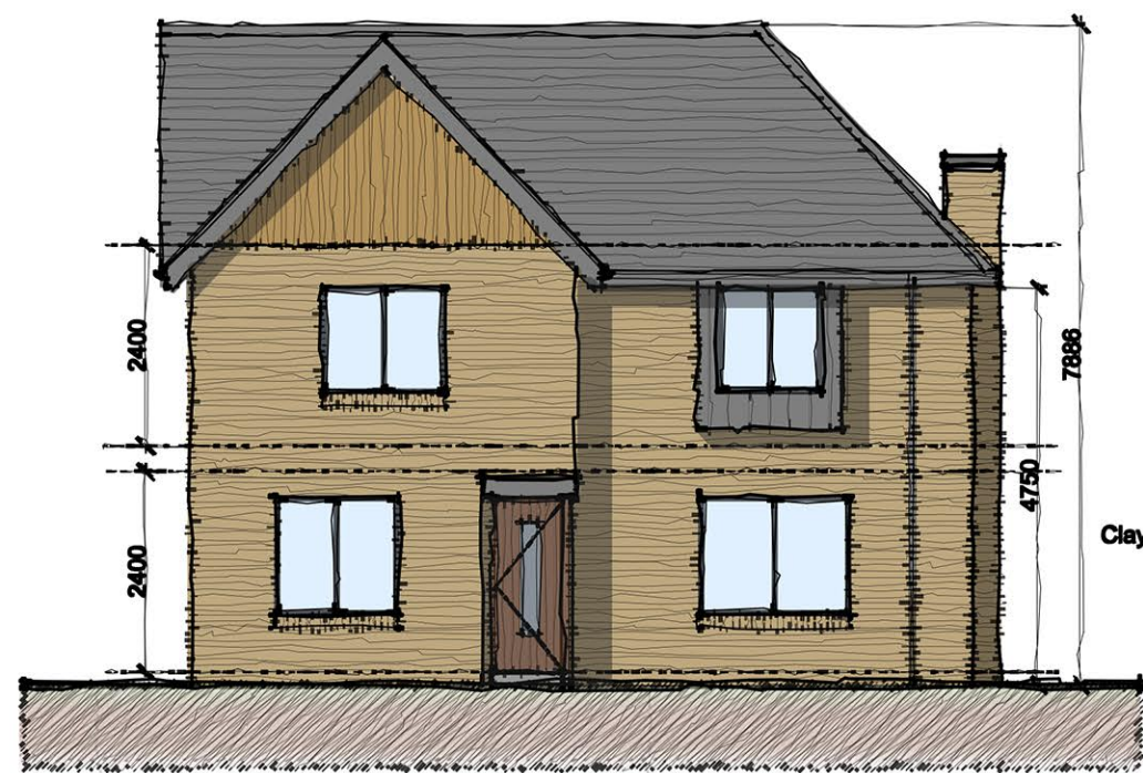
Proposed Front Elevation (South) Scale 1:100
