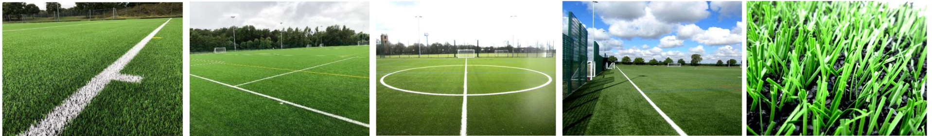
3G synthetic turf surface, its appearance similar to well-maintained natural grass
