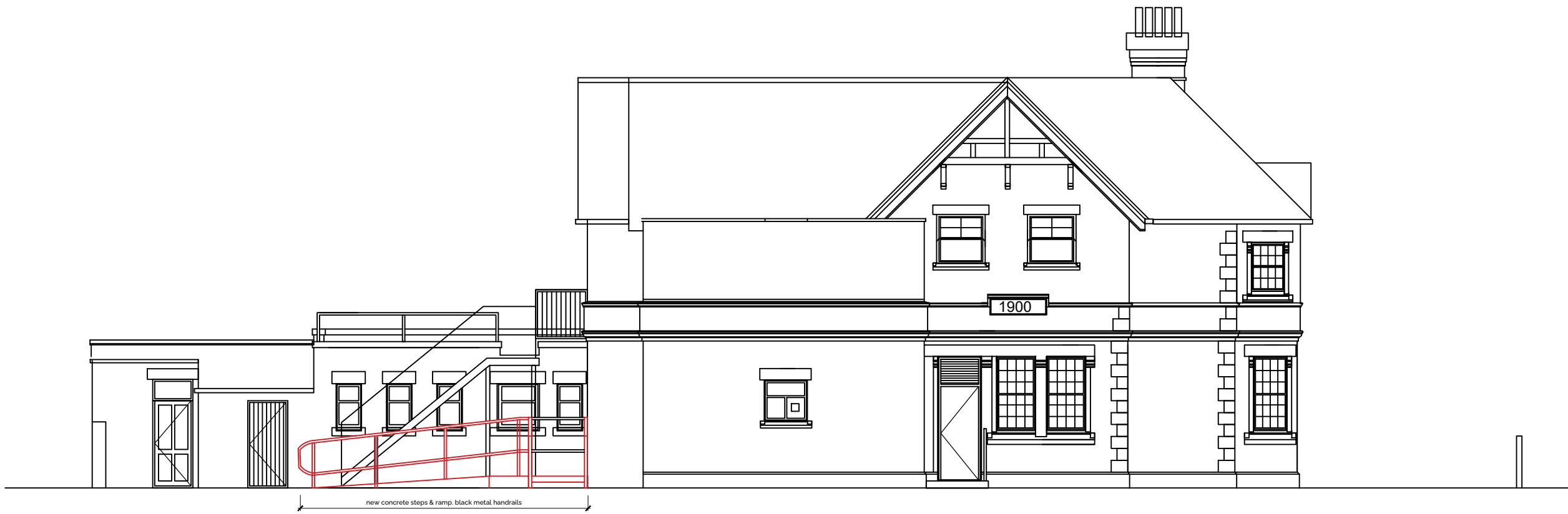
SIDE ELEVATION - ramp detail Scale 1:100
