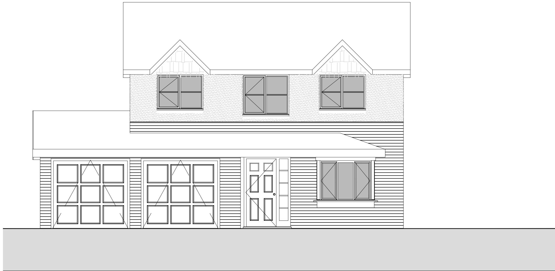
EXISTING FRONT ELEVATION 1:50
