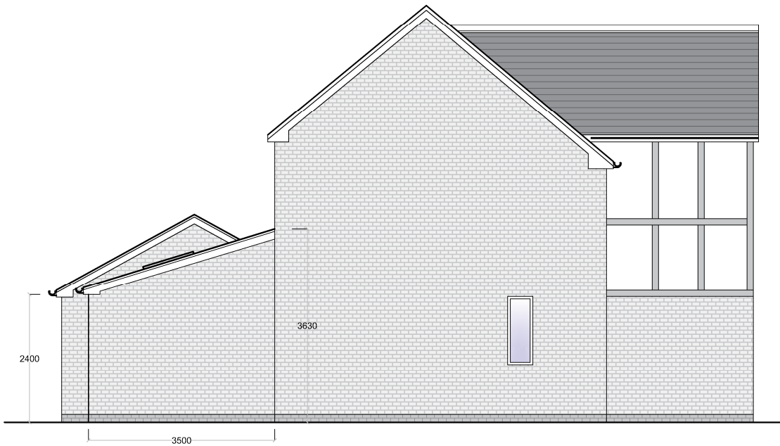
PROPOSED SIDE ELEVATION (Scale 1:100) SCALE BAR - (mm) 500 1000 2000
