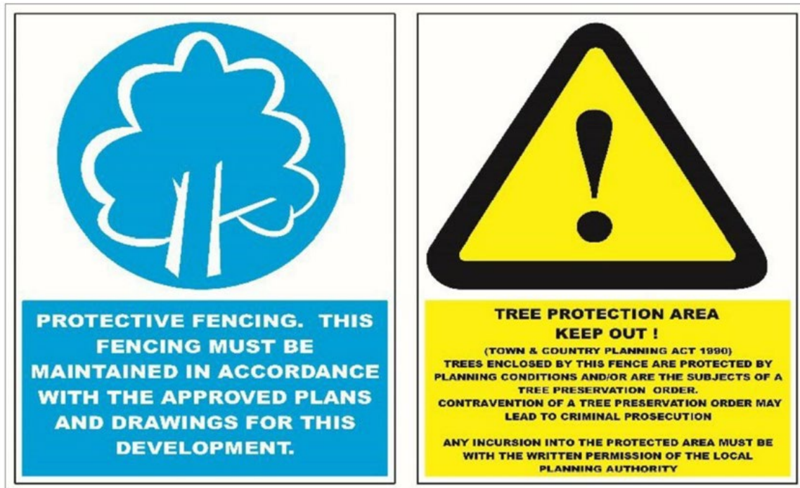
Figure 1. Tree protection notice to be fixed to protective fencing
