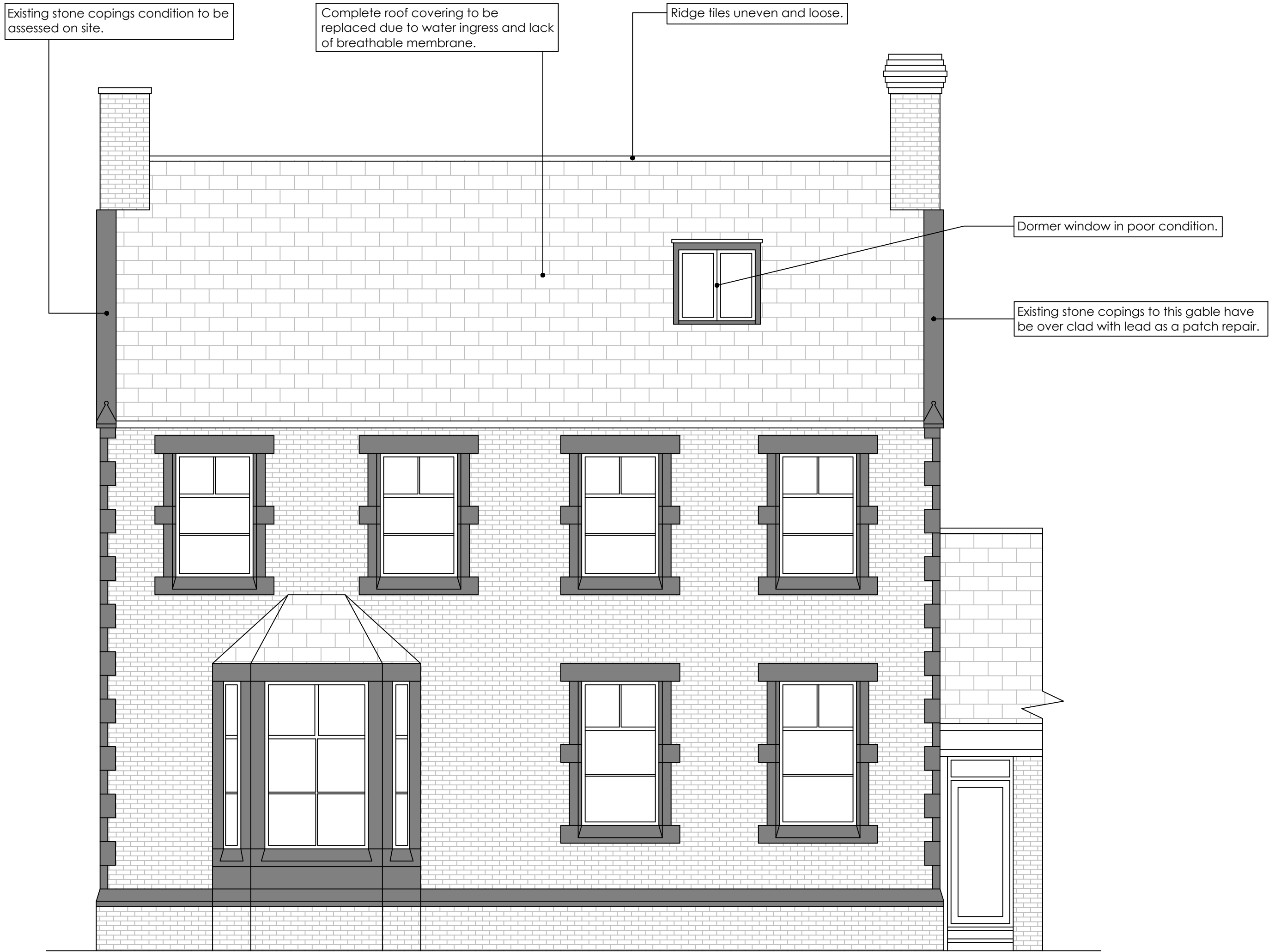
1 SOUTH ELEVATION AS EXISTING SCALE | 1:50
