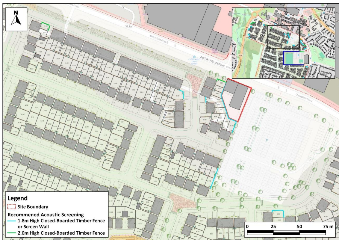
Figure 8.3.7: Recommended Acoustic Screening [2]
