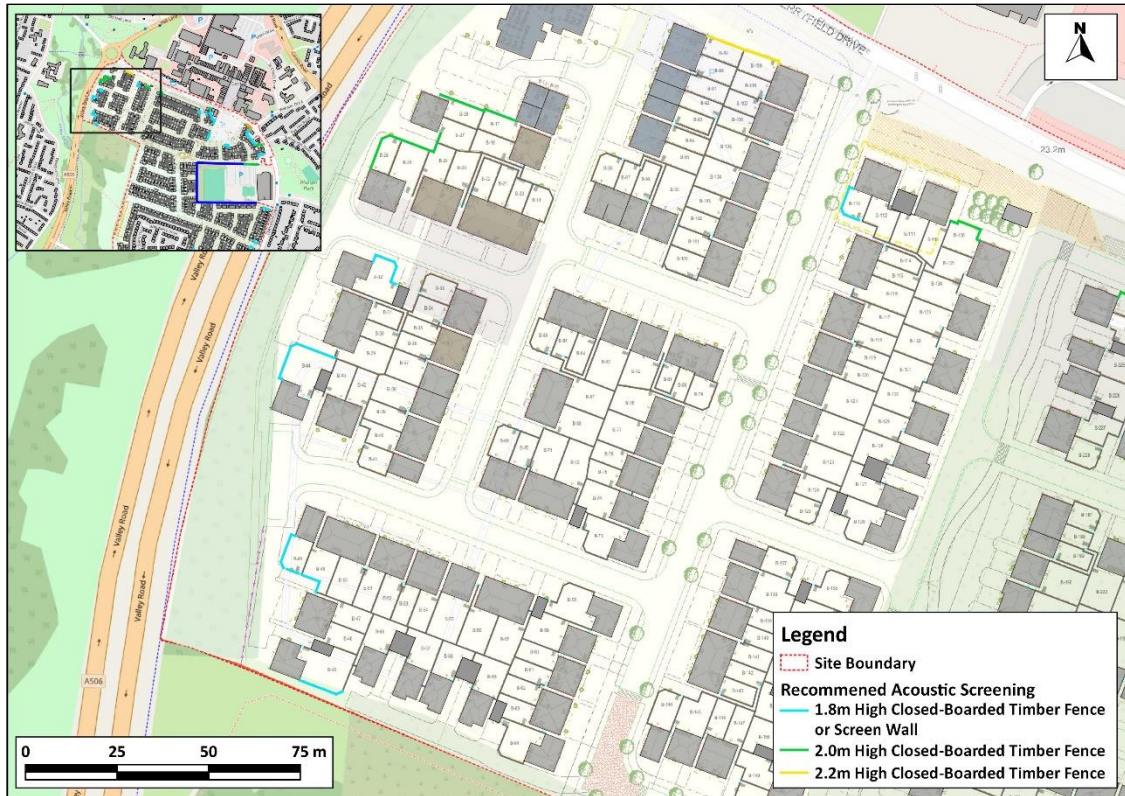
Figure 8.3.6: Recommended Acoustic Screening [1]
