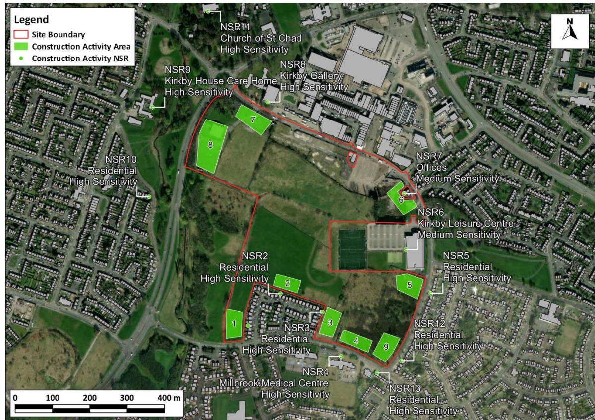
Figure 8.1: Construction Activity Areas and Noise Sensitive Receptors
