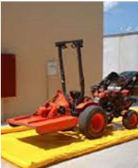
Figure 17. Example of type of LOCALISED wheel wash enclosure to be used
