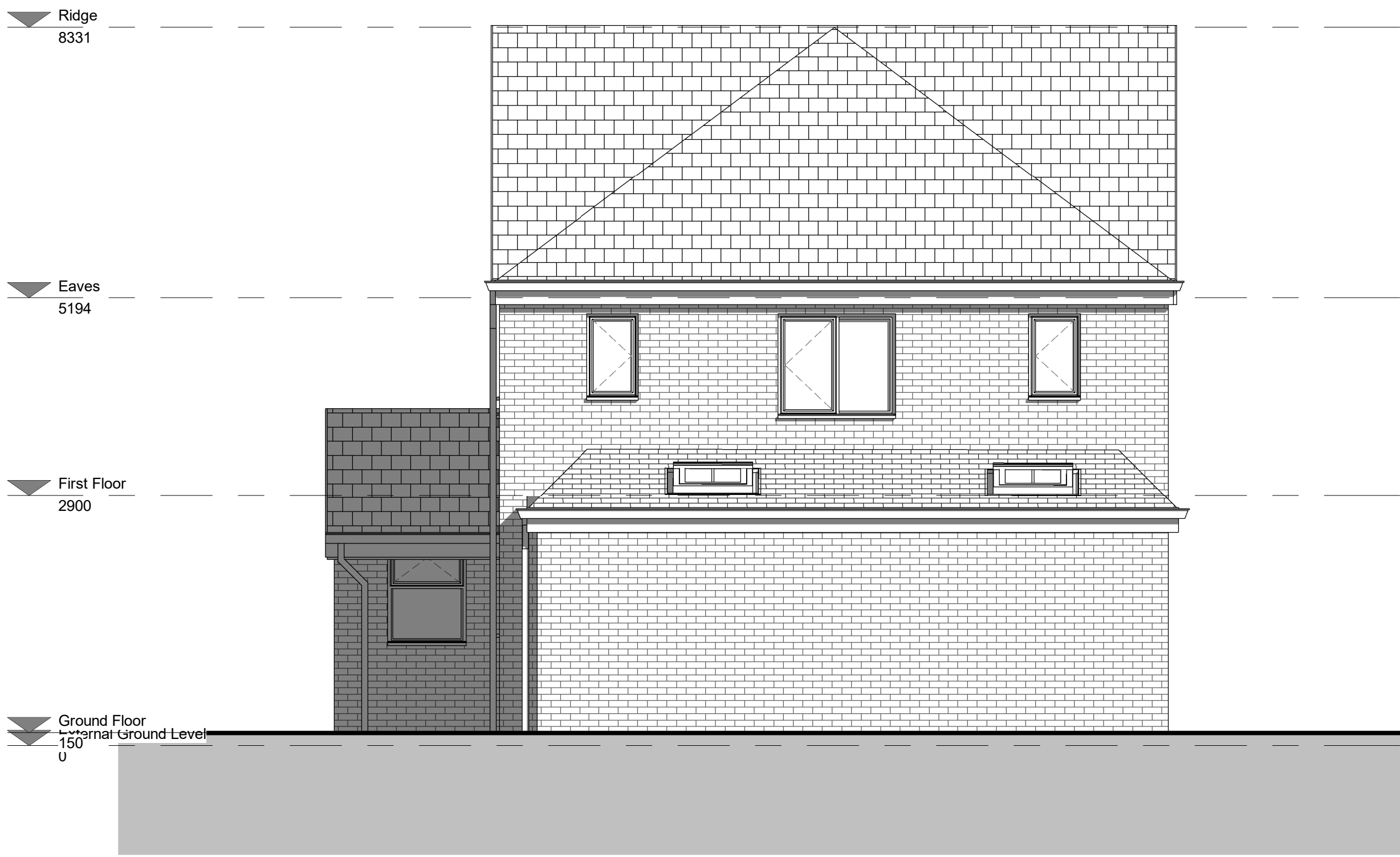
4 Proposed Right Elevation 1 : 50
