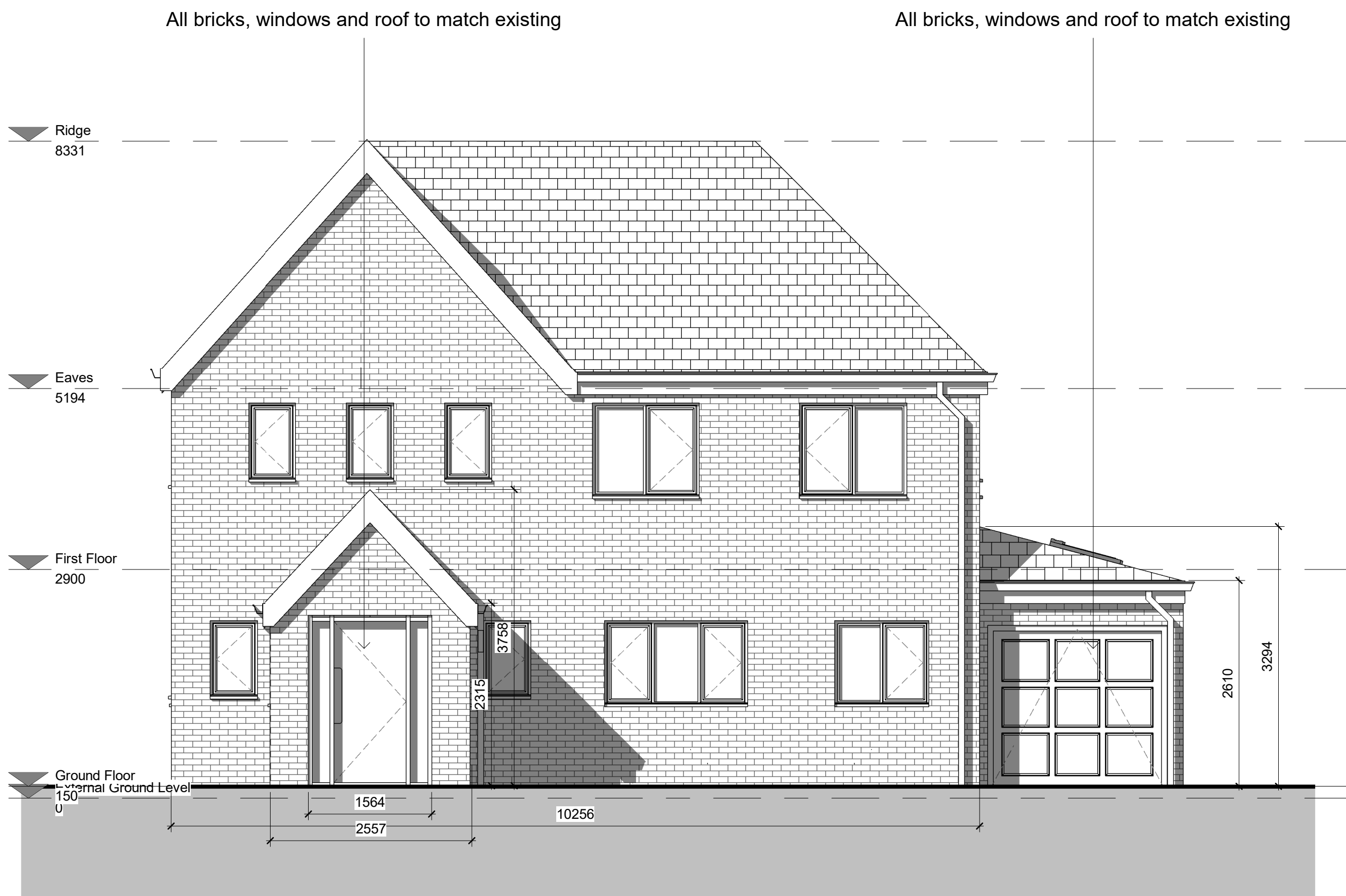
3 Proposed Front Elevation 1 : 50
