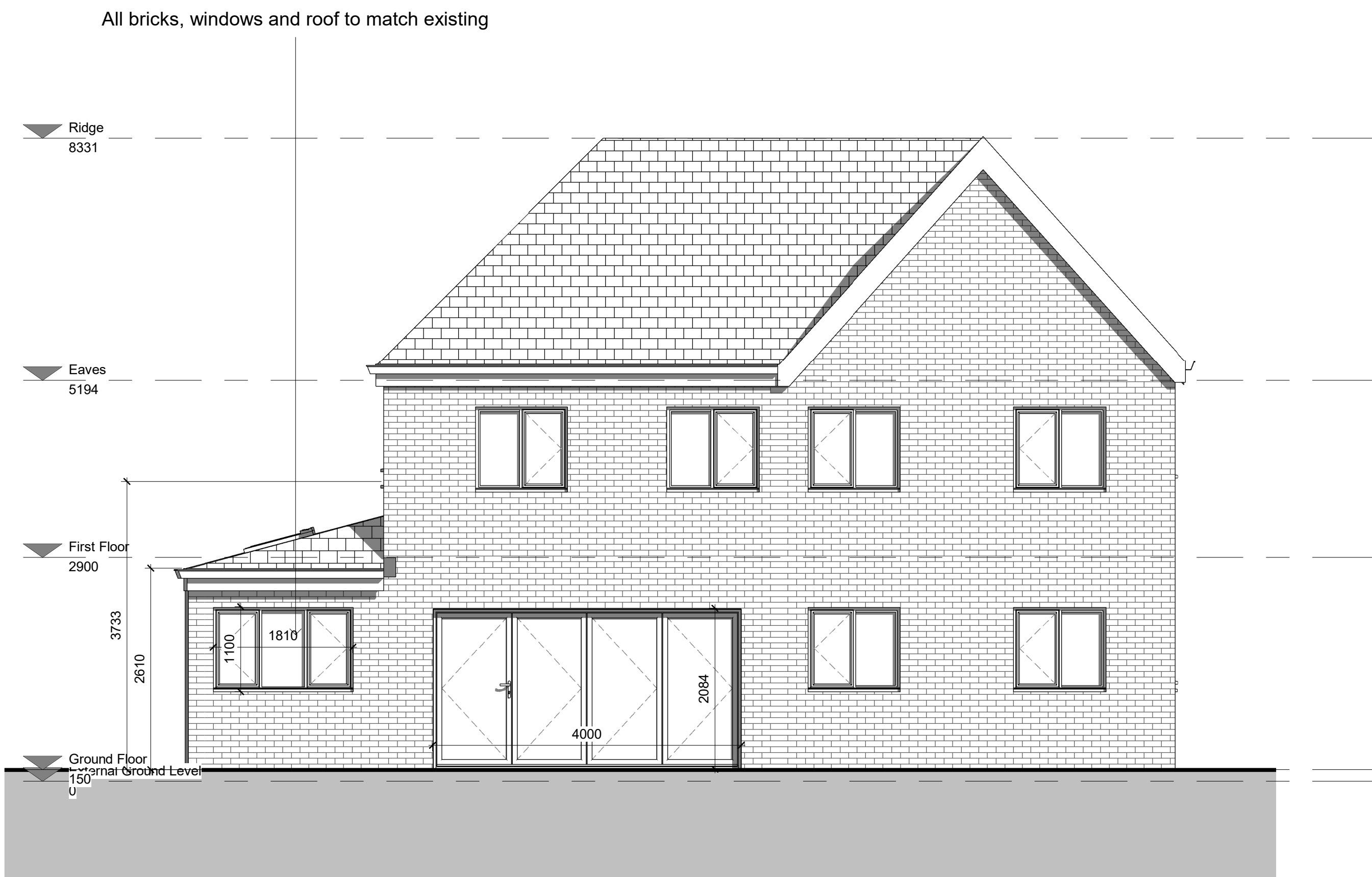
4 Proposed Rear Elevation 1 : 50
