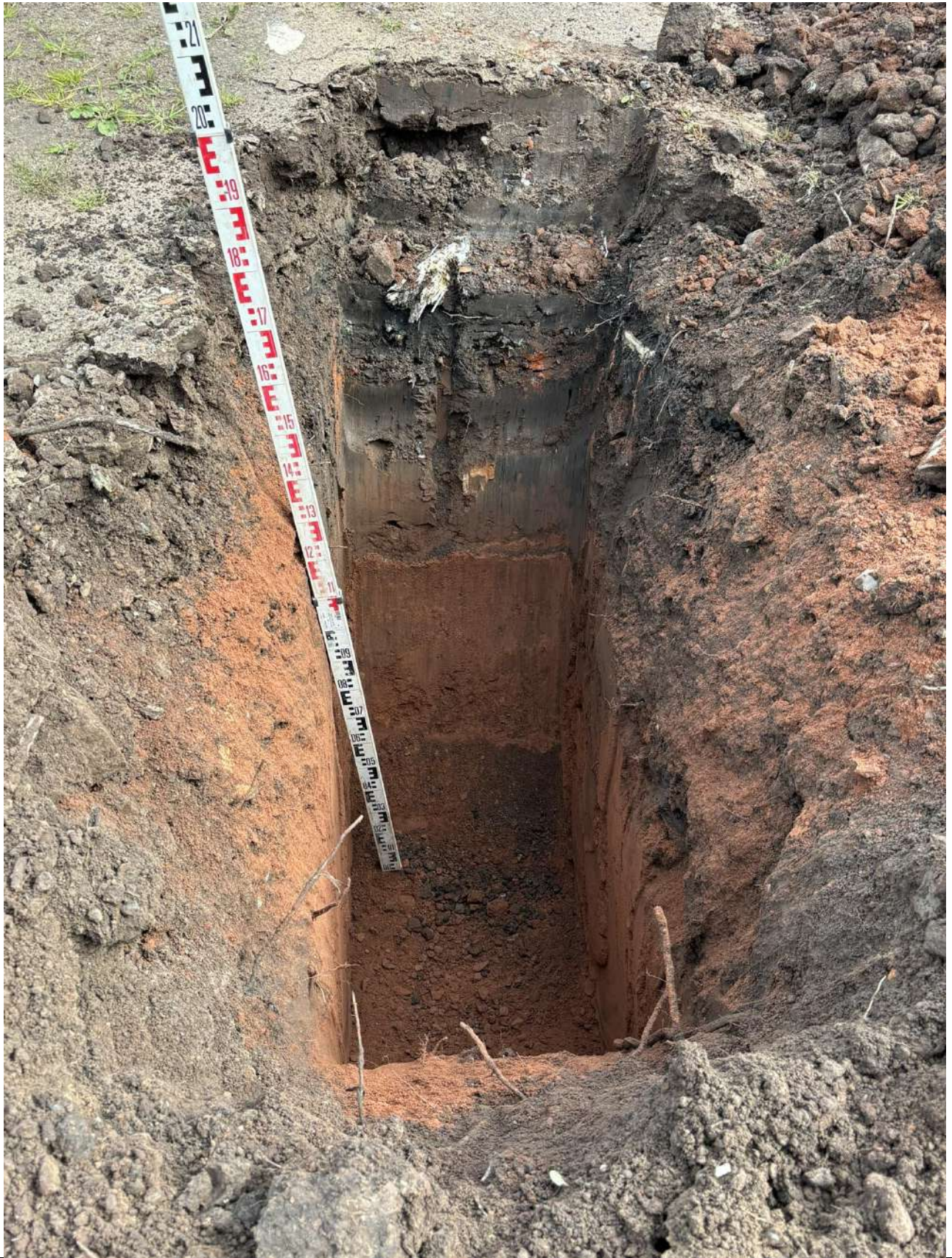
Plate 12: TP12 showing northern face and the base of the excavation
