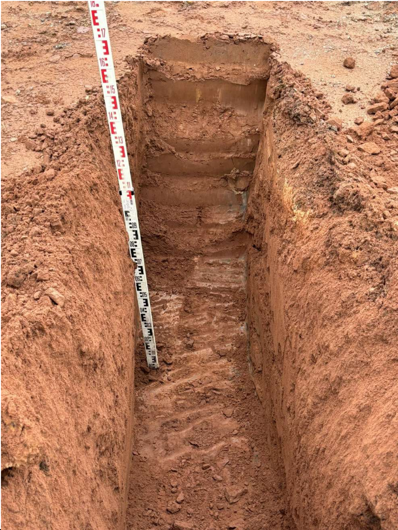
Plate 3: TP03 showing the base of excavation and vertical side wall of pit
