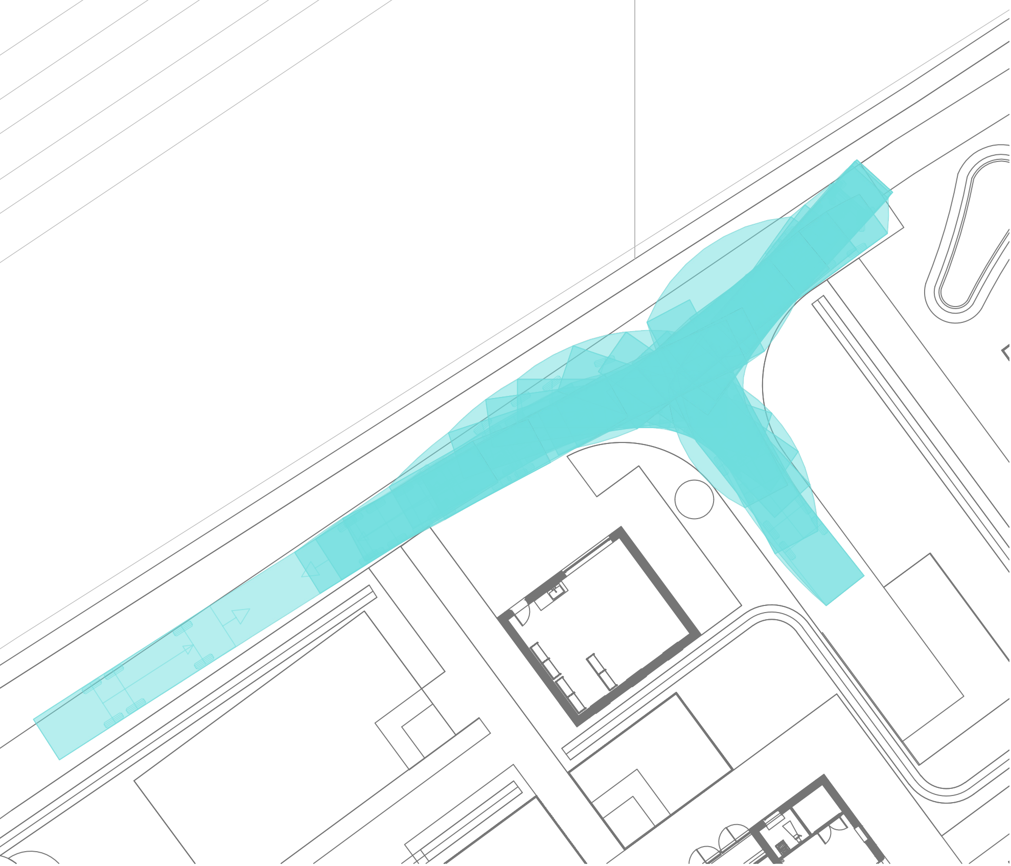
Refuse Vehicle Internal Turning Head
