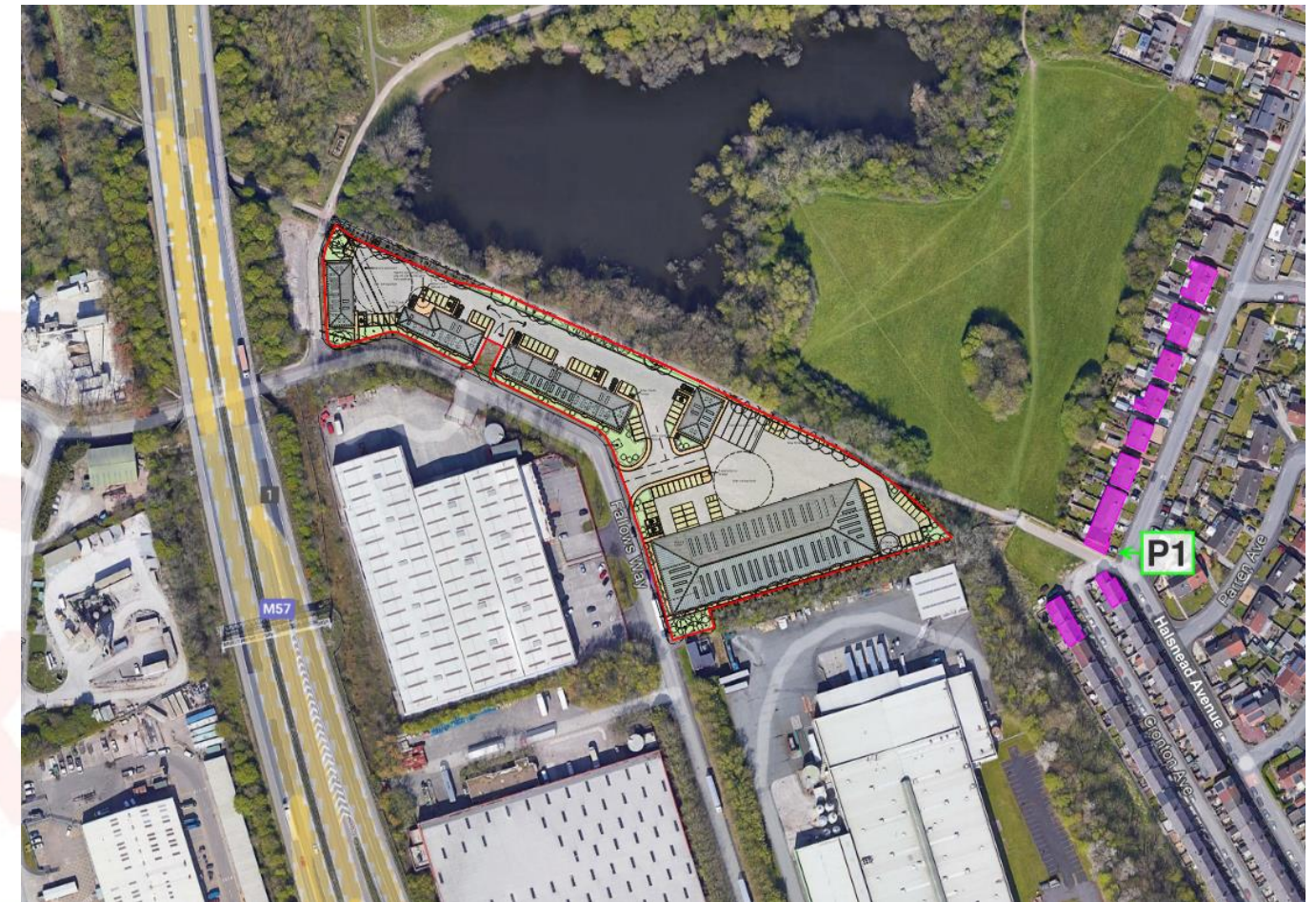
Figure 1: Extract from the proposed site plan overlaid on an aerial image of the site with site boundary (red), unattended 24-hour noise measurement position P1 (green) and nearest identified noise-sensitive receptors (NSR)(pink)
