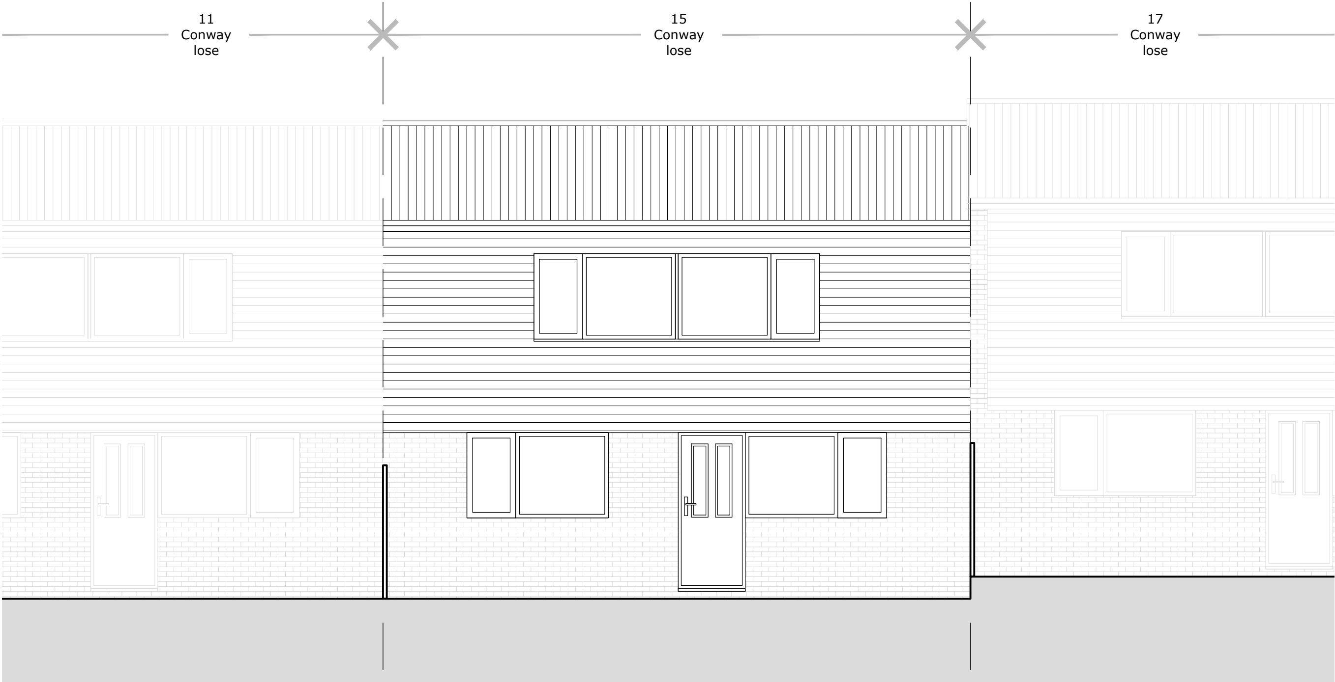
South Elevation as PROPOSED 1:50
