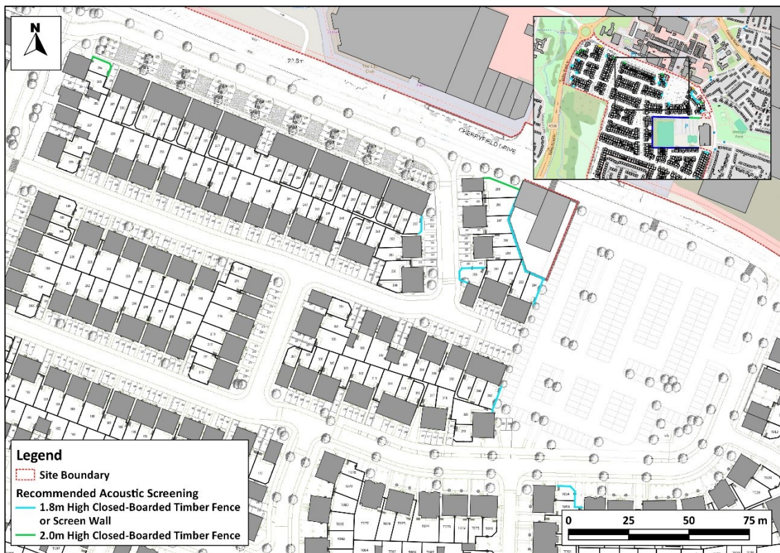
Figure 8.3.7: Recommended Acoustic Screening [2]
