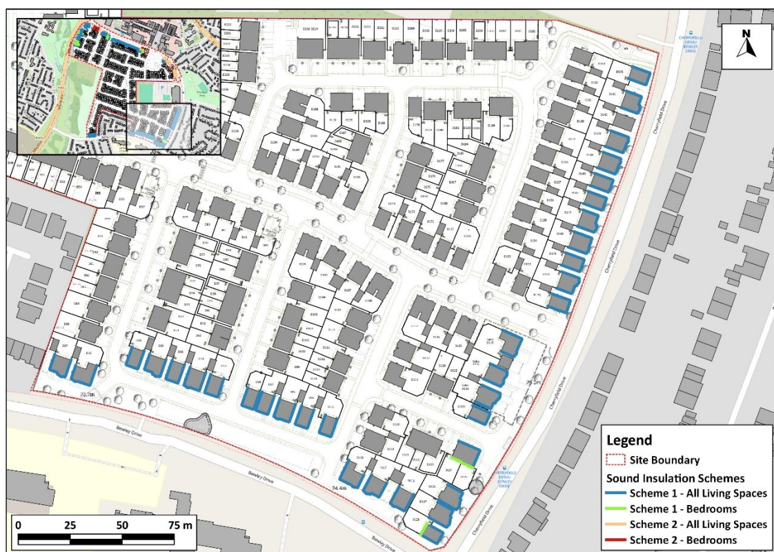
Figure 8.3.14: Recommended Road Traffic Sound Insulation Scheme [4]
