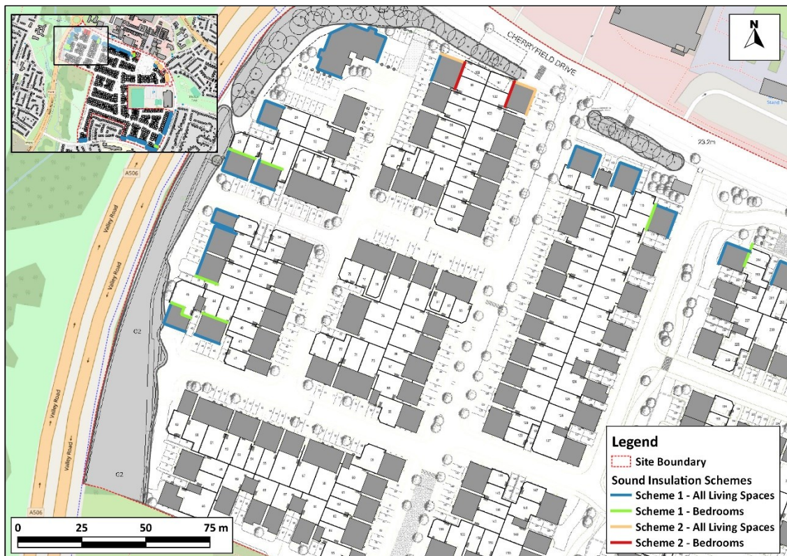
Figure 8.3.11: Recommended Road Traffic Sound Insulation Scheme [1]
