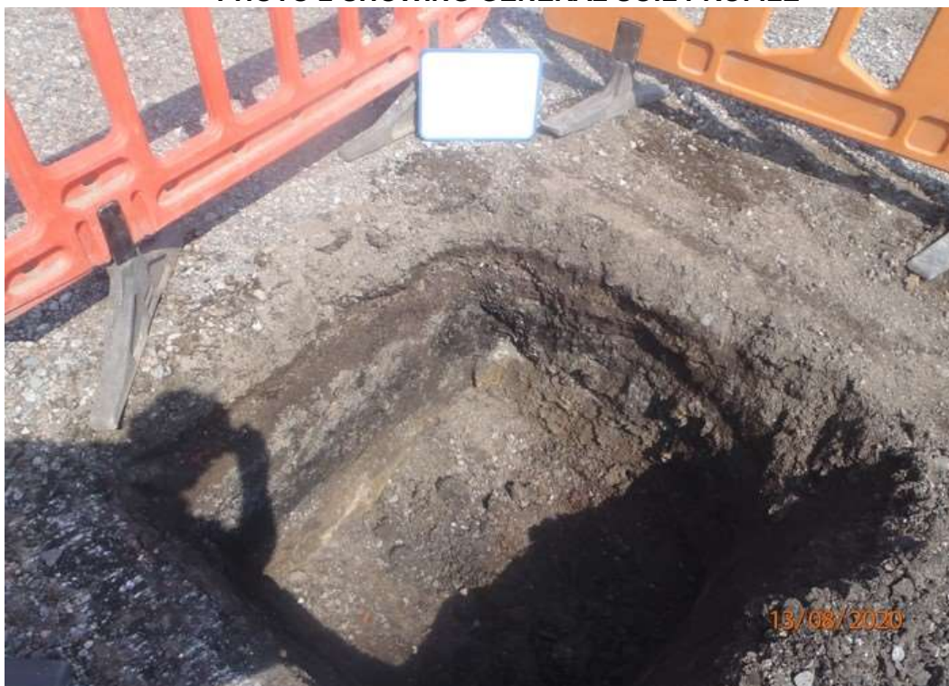
PHOTO 2 SHOWING GENERAL SOIL PROFILE
