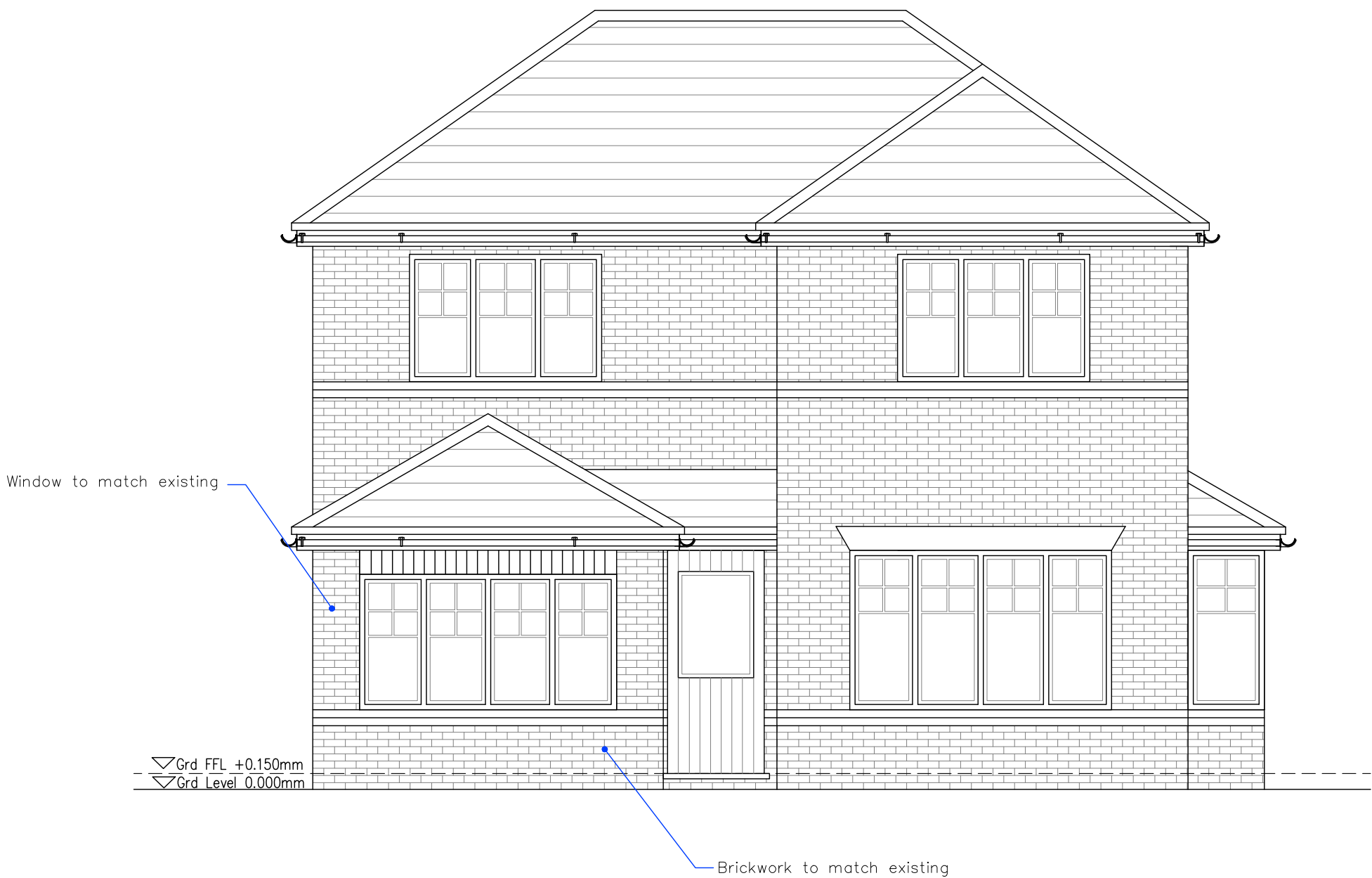
PROPOSED FRONT ELEVATION | SCALE 1:50
