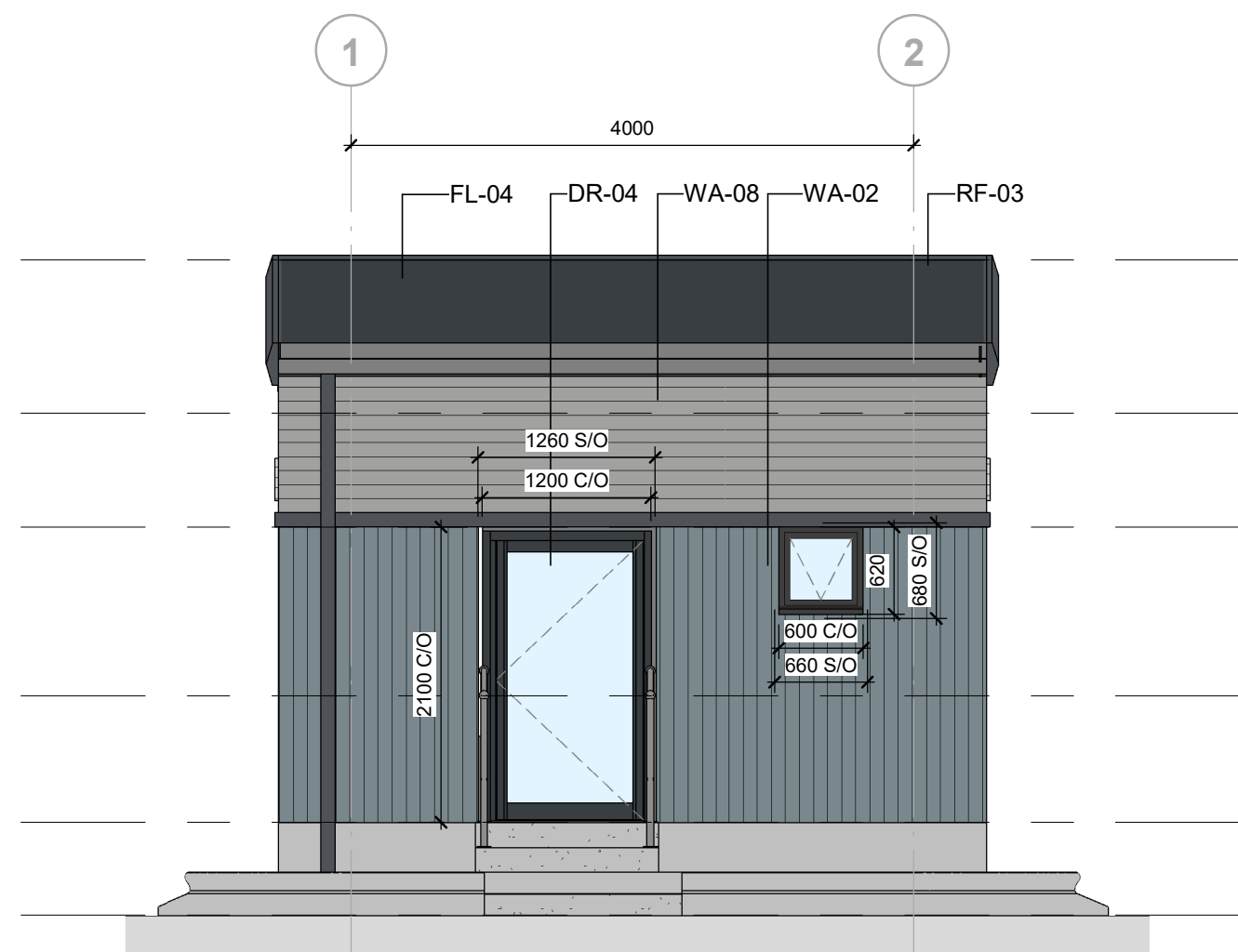
North West Elevation 1 : 50
