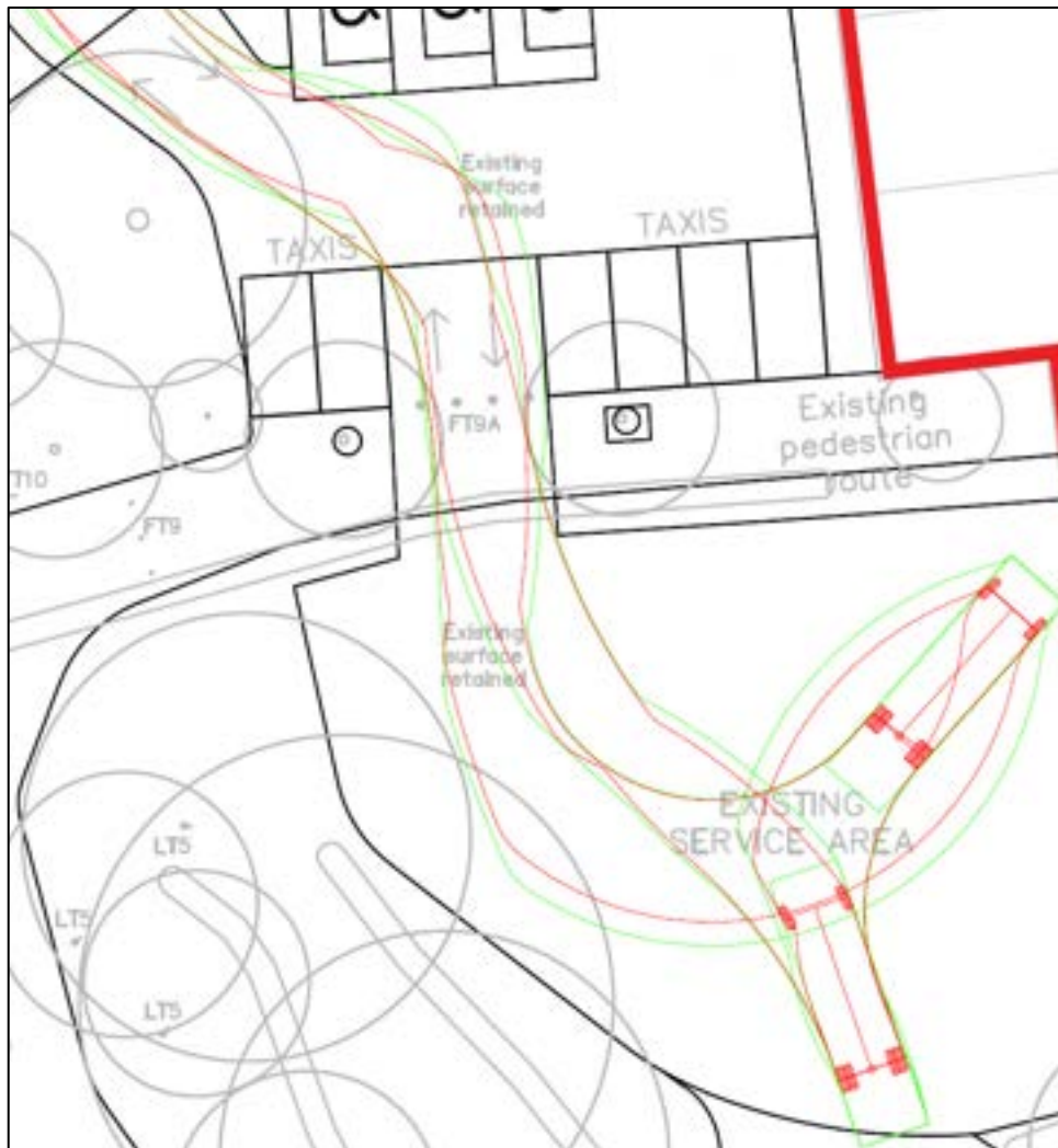
Figure 5.12: Vehicle Tracking of 10m Rigid HGV for the Servicing Area to the South of Cavendish House
