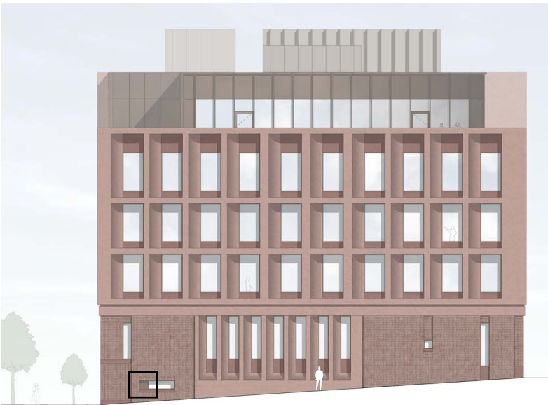
Southwest elevation: areas of patterned perforated metal
