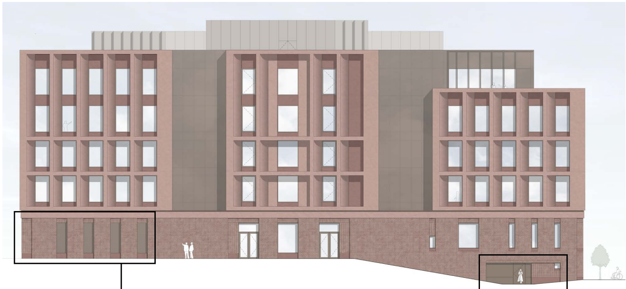
Northwest elevation: Archway Road, areas of patterned perforated metal
