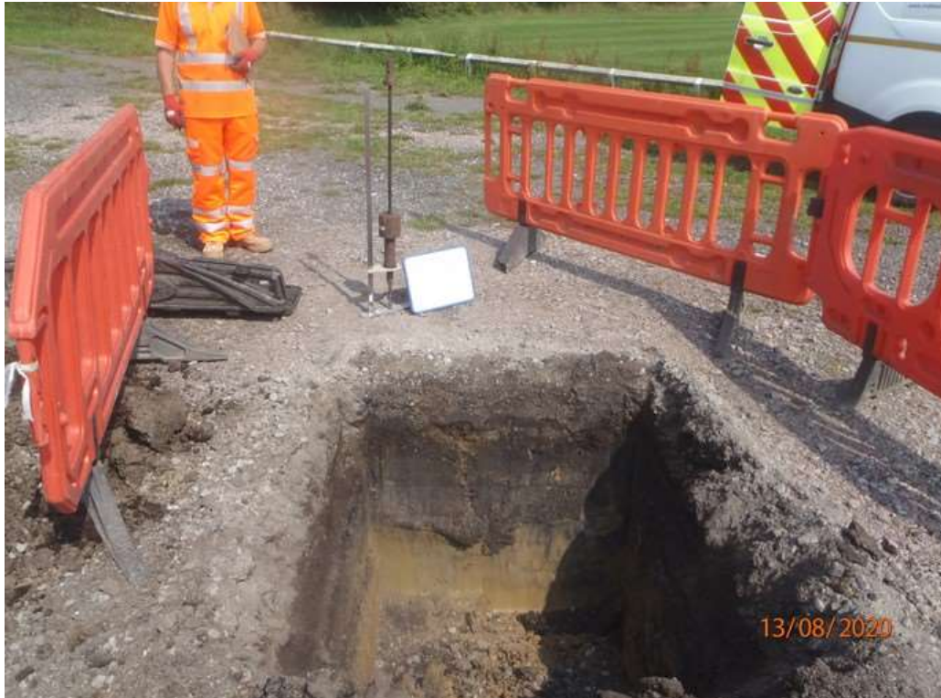
PHOTO 6 SHOWING SOAKAWAY LEVEL ON 2nd DAY
