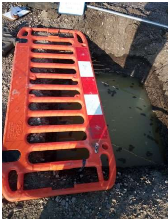
PHOTO 6 SHOWING SOAKAWAY LEVEL ON 2nd DAY
