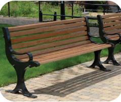
The Broxap 'Blackburn Seat' (or equivalent) or bespoke seating. Cast iron frame seat in streamlined contemporary design with eleven treated hardwood slats. Fixing: Root fixed Dimension: L1800 x W605 x H840 mm Material: Engineering grade 250 Cast iron and hardwood Colour: Black (RAL 9005) Finish: Treated hardwood. Cast iron finished with a primer undercoat and a 2 - pack acrylic topcoat Extras: Embellishments painted white
