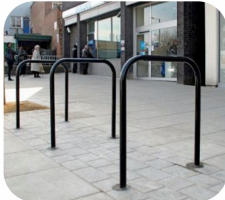
The Broxap 'Sheffield Cycle Stand' (or equivalent). This simple hoop design allows cycles to be secured to the continuous one-piece steel tube in a variety of ways. Fixing: Root Fixed Dimension: W715 x H800 x DIAM48.3 mm Material: Galvanised steel Colour: Black (RAL 9005) Finish: Polyester Powder Coated Extras: Other sizes available
