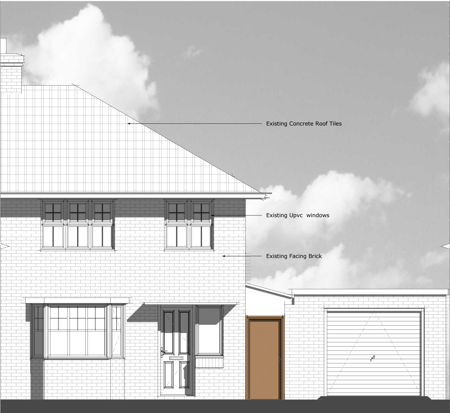
02 Existing Front Elevation
