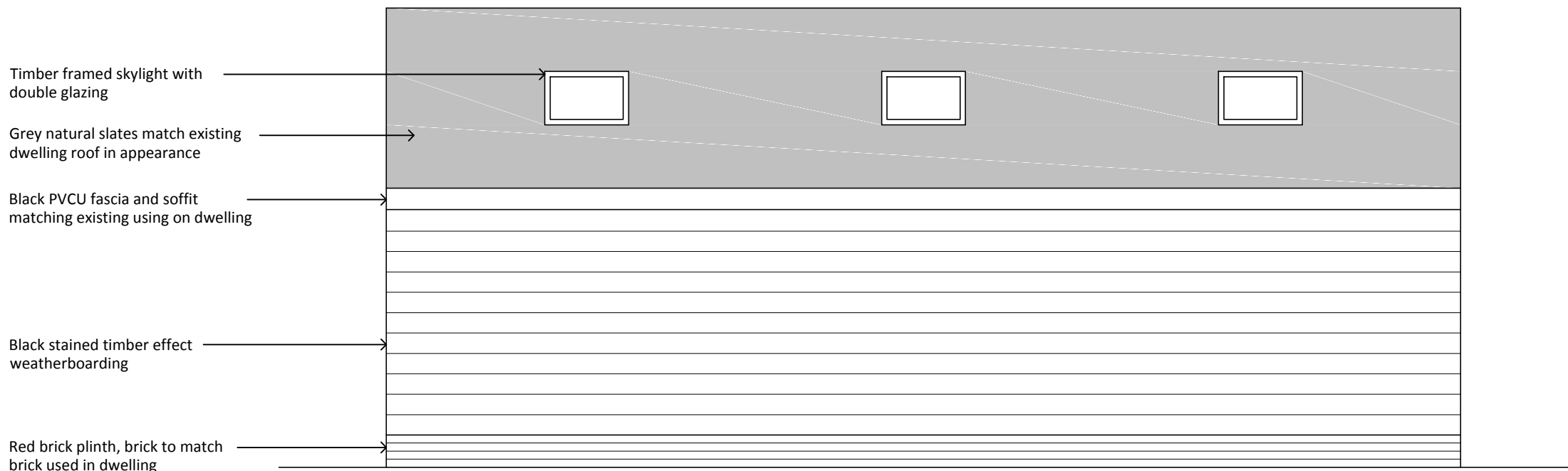
PROPOSED REAR ELEVATION - NORTH SCALE 1:50
