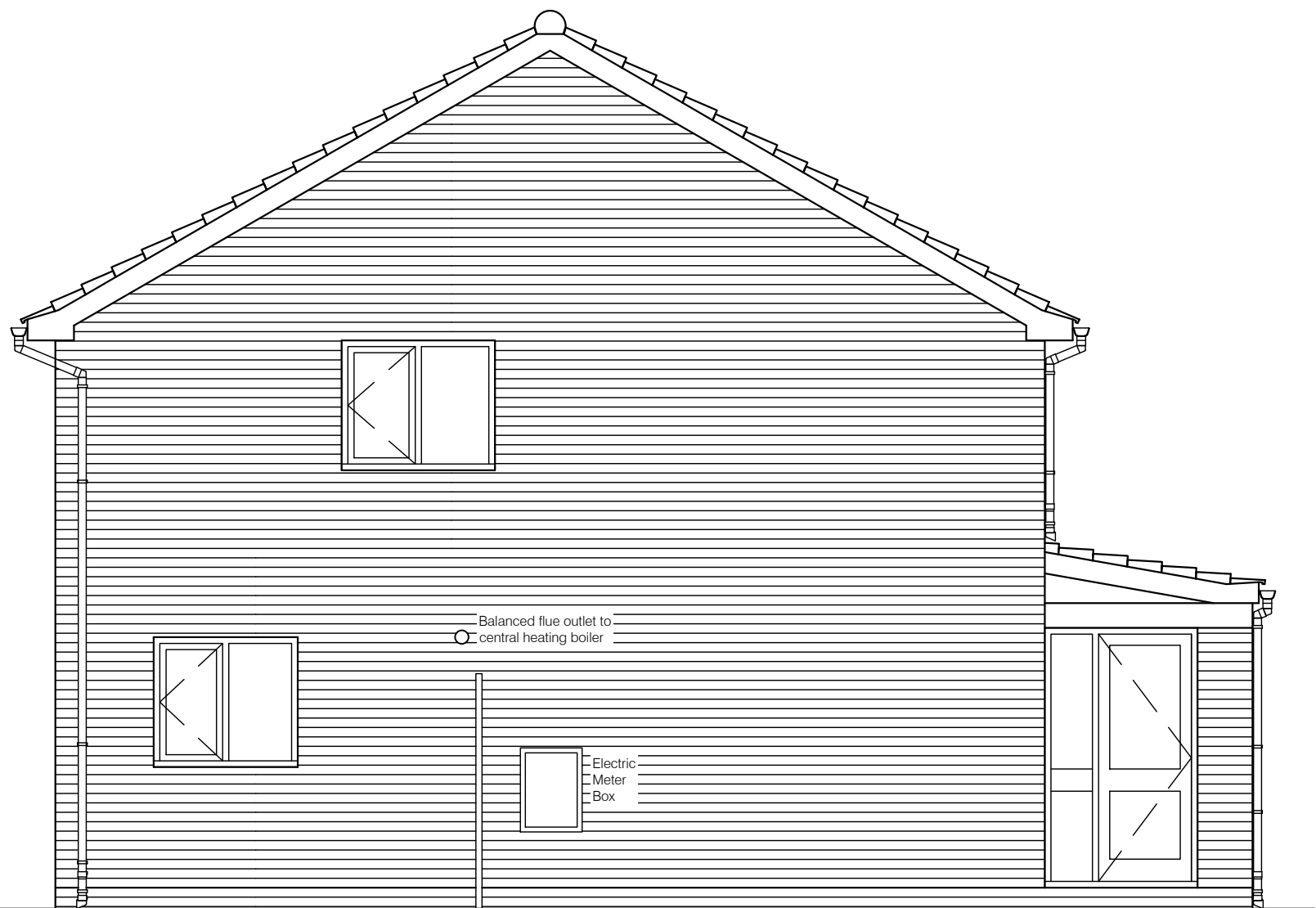
GABLE (SIDE) ELEVATION
