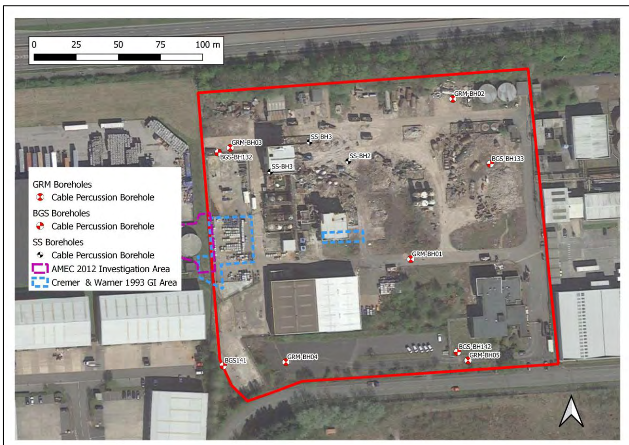
Figure 2.4 Selected previous exploratory holes
