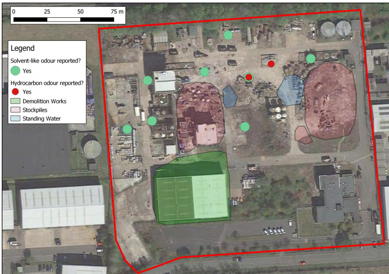
Figure 4.3 Evidence of Contamination
