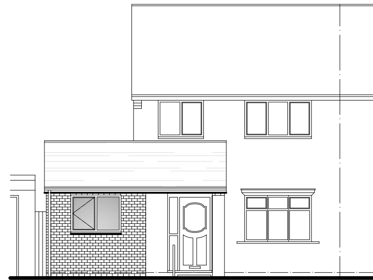
Proposed front elevation @ 1:100 scale
