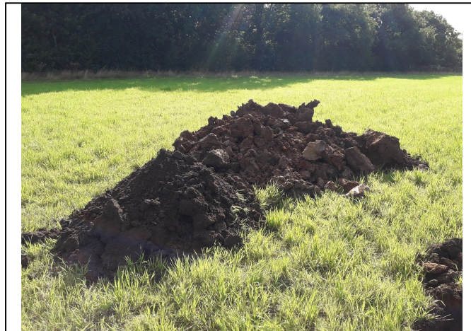
Trial Pit 103 Spoil
