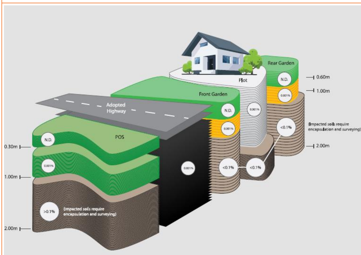
FIGURE 4.1 ASBESTOS RISK MITIGATION CONCEPTUAL SITE MODEL
