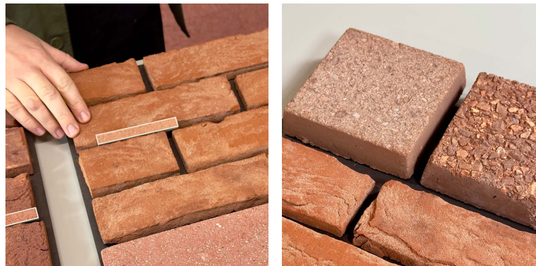
Samples: Light & dark 'sandstone' reconstituted stone, red brick stocks, grey/bronze powder coated aluminium
