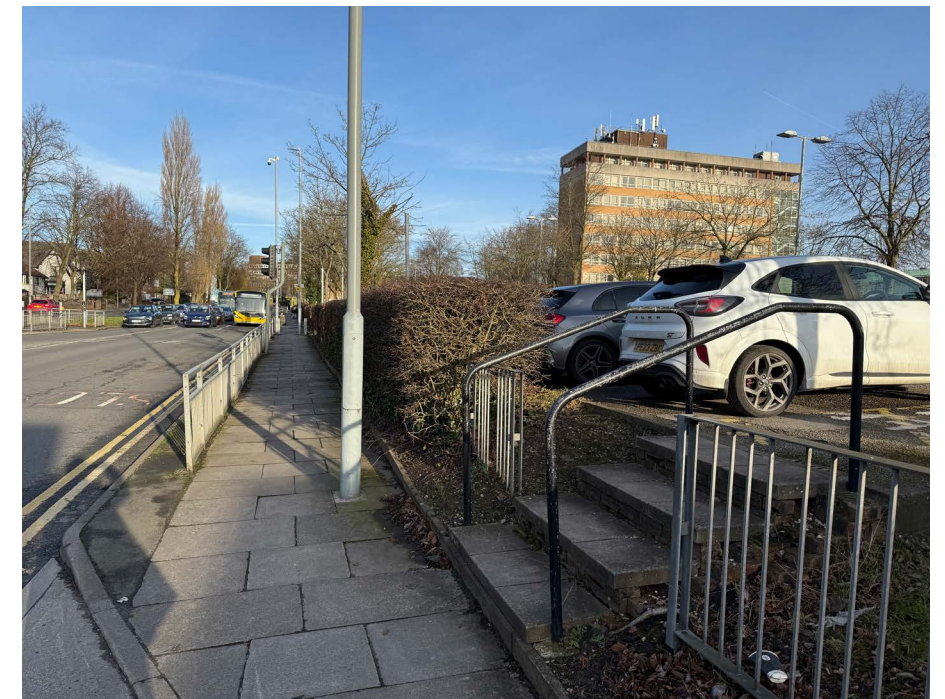
Figure 2.58: Level changes with no accessible alternative route and narrow pavements make for a challenging environment to navigate.
