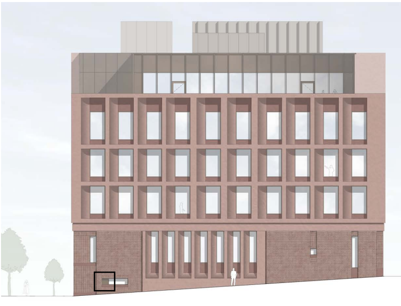
Southwest elevation: areas of patterned perforated metal
