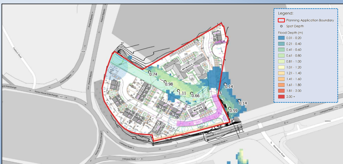
Figure 9: Proposed Fluvial 1 in 100yr plus 44% CC with 95% Blockage Flood Depth Extract (Betts Hydro, 2022)
