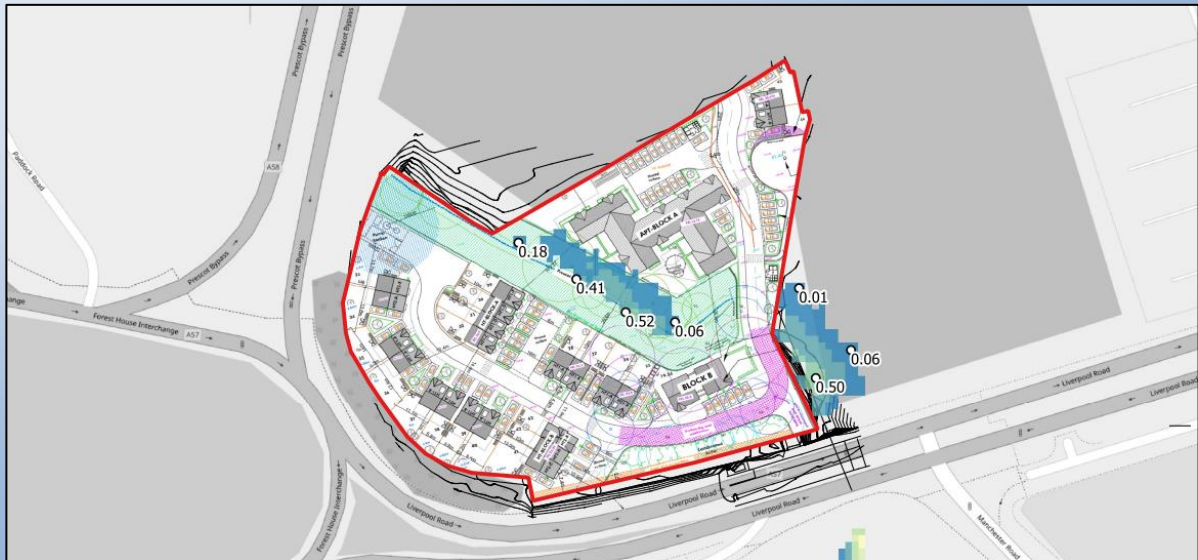
Figure 8: Proposed Fluvial 1 in 100yr plus 44% CC Flood Depth Extract (Betts Hydro, 2022)
