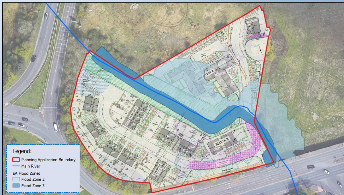
Figure 4: EA Flood Zone Overlay Plan Extract (Betts Hydro, 2022)
