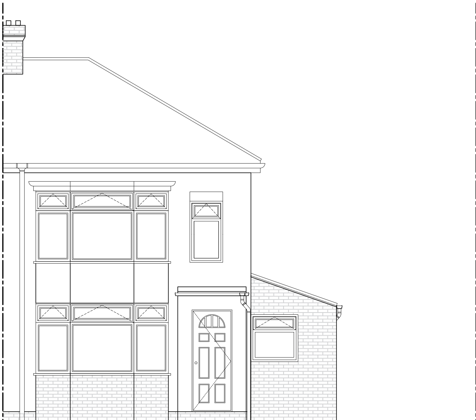
① Existing front elevation
