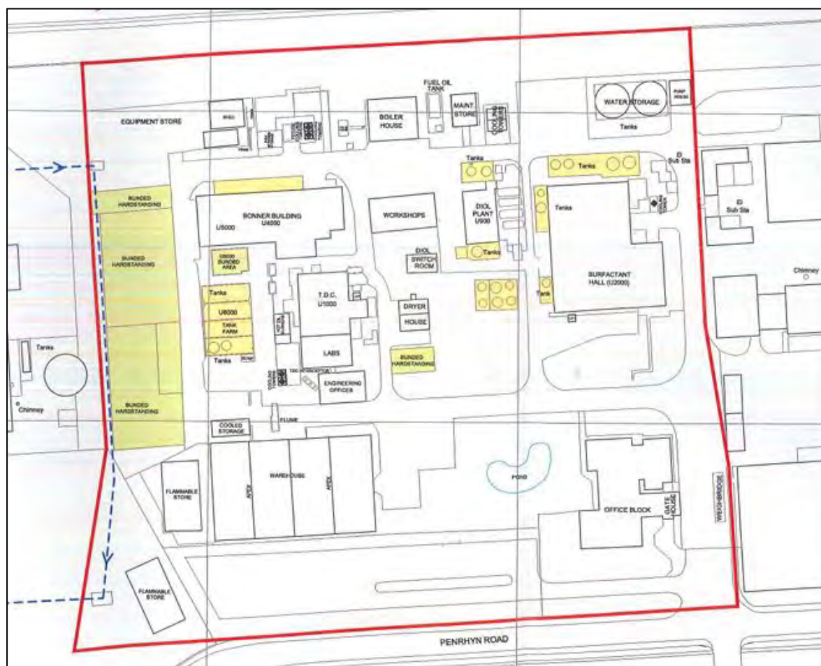
Figure 2.2 Former Chemical Works Layout
