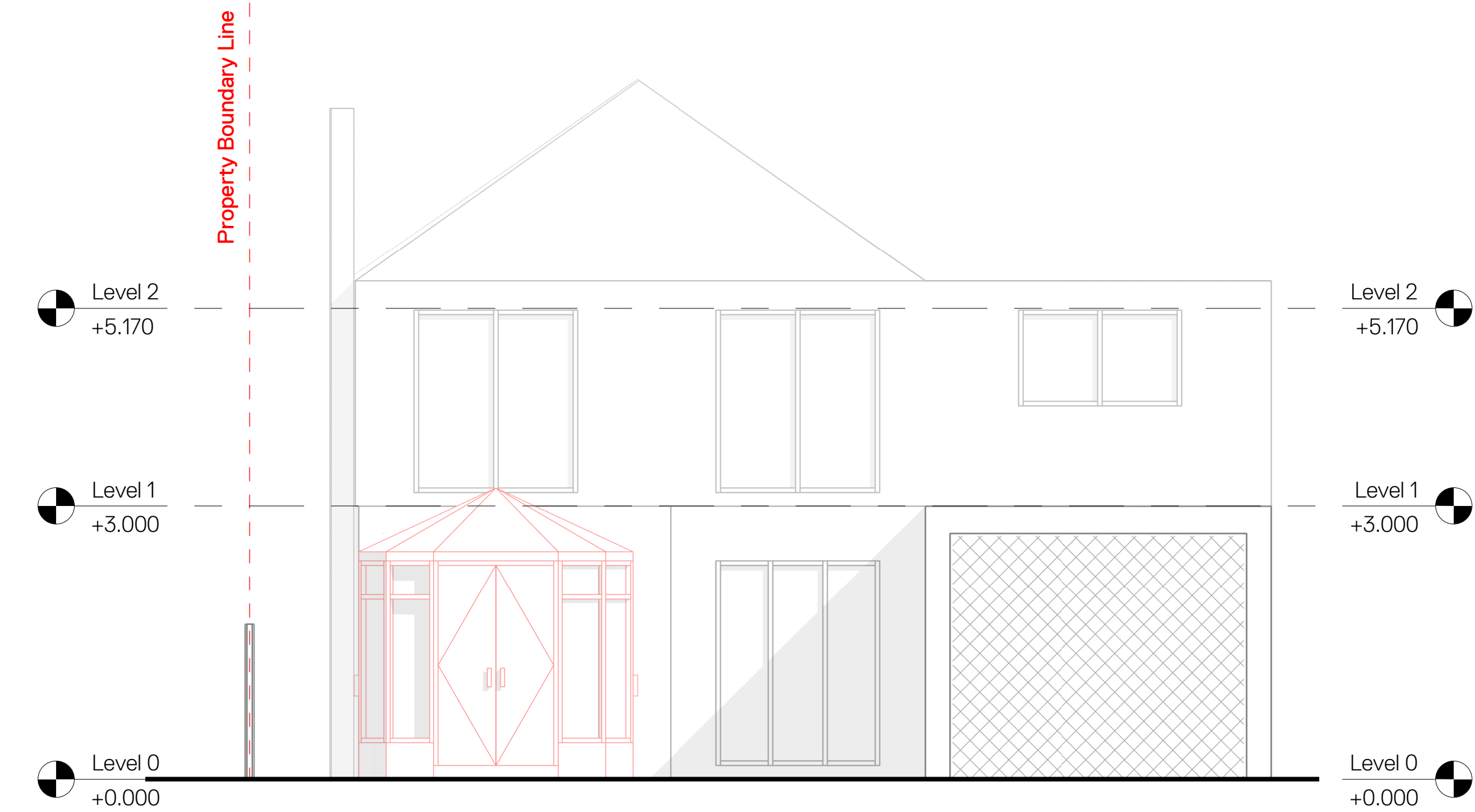
1 Demolition Garden Elevation 1 : 50
